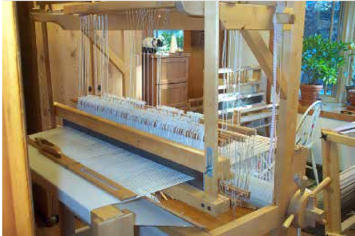
First floor loom - Lilqvist from Finland 8 shafts/8 treadles
