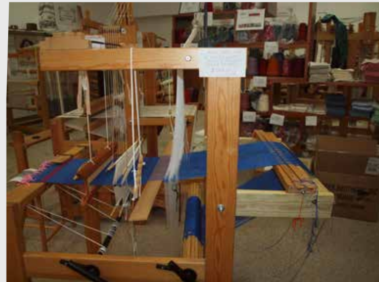
Julia loom, modified, with Lao fuum (reed/beater, pre-threaded heddles on two shafts, pre-threaded vertical pattern storage for patterning)
