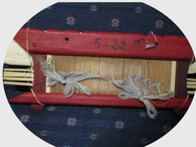
Lao „fuum“ – insert into loom and weave. pre-sleyed reed/beater, pre-threaded shafts, pre-threaded pattern heddles
