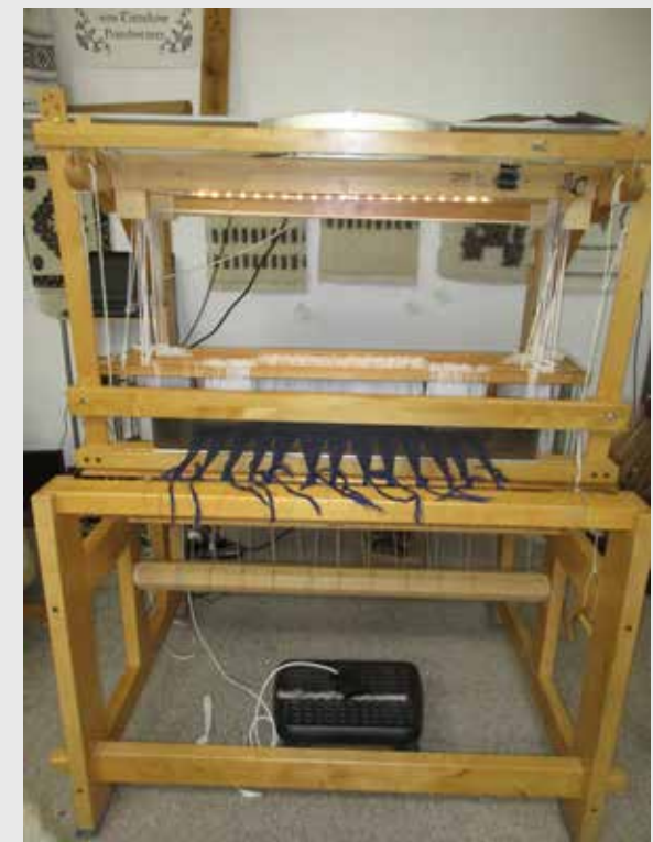
Original Lilqvist loom with Toika dobby mounted computer assisted operation with foot pedal
