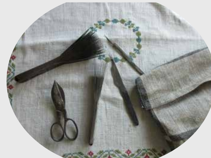
Tools for knotted pile weaving – all hand forged Lg and sm beaters, pile shears, hook knives for cutting knots
